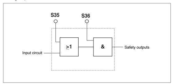
Logic inputs S35 and S36 from the PNOZ e1.1p enable additional PNOZelog or PNOZmulti units to be logically AND/OR connected.
